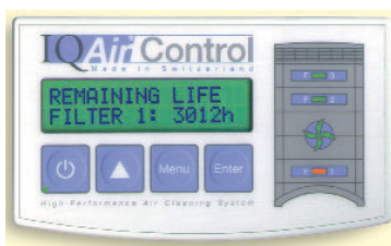
LED on the control panel turns red when it's time to change a filter
