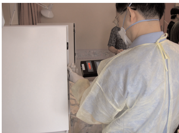
Mark Lau of the EMSD testing the actual filtration efficiency of a non-certified air cleaner with a laser particle counter. The majority of air cleaners failed the test.
