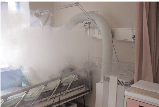
Testing the IQAir® in location. Artificial smoke is generated on a hospital bed and then captured at source with the help of the IQAir® FlexVac's flexible suction arm.
